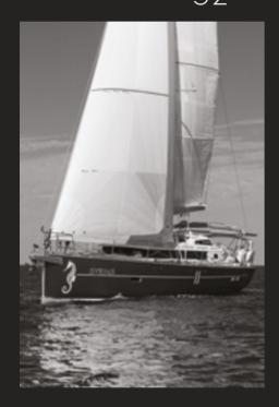
Length overall 16,65 m 4,80 m Beam 2,90 m Draught (centreboard down) Draught (centreboard raised) 1,27 m Air draught (excluding antennas) 21,50 m Displacement (est.) 19,5 t Ballast 6,57 t Upwind sail area 120.5 m<sup>2</sup> Gennaker/Spinnaker 130 m<sup>2</sup> / 186 m<sup>2</sup> 110 CV Engine Diesel capacity (est.) 1 200 l Water capacity (est.) 880 I Number of cabins 3-4 Number of berths 5-6-8
