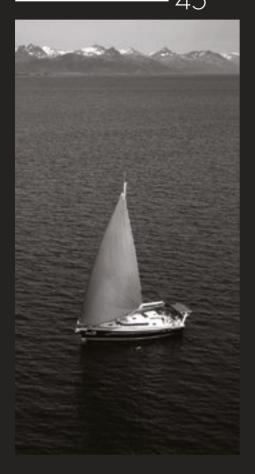
Length overall 14,88 m Beam 4,44 m 2,90 m Draught (centreboard down) 1,14 m Draught (centreboard raised) Air draught (excluding antennas) 19,80 m Displacement (est.) 14,61 t Ballast 4,54 t Upwind sail area 91 m<sup>2</sup> Gennaker/Spinnaker 90 m<sup>2</sup> / 160 m<sup>2</sup> 75 CV Engine Diesel capacity (est.) 700 I Water capacity (est.) 500 I Number of cabins 2-3 Number of berths 5-6-8
